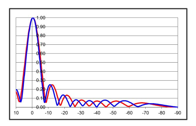
Here is the elevation plot of the two stations. 96 MHz is the RED plot, and 104 MHz is the BLUE plot. The radiation from the main beam is very close for both stations. As a bonus the radiation from -50 to -90 degrees is about 10 dB lower than a standard full wavelength-spaced antenna. The vertical space needed to mount the antenna has been reduced compared to a full-wave spaced antenna. The elevation gain however is slightly lower as a function of bay-count for the short spaced antenna.
